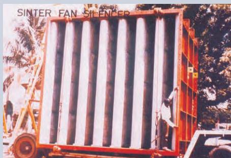
The discharge silencer having a dimension of 4200mm wide x4050mm height x 3300mm length weighing 14MT being dispatched from our factory.
